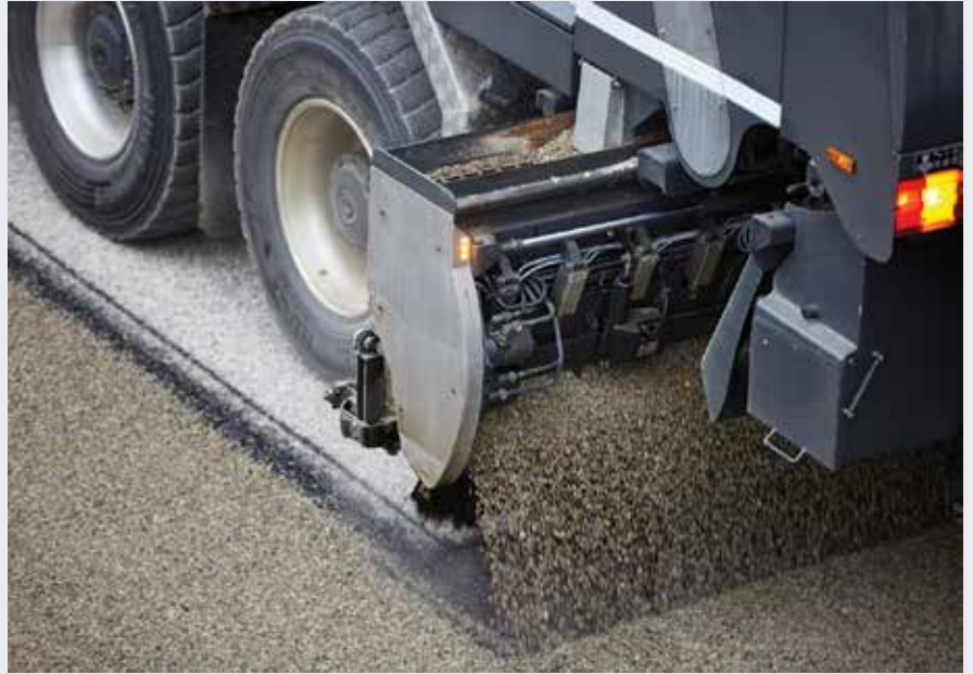
The AMS Road Sealer from Asphalt Maintenance Solutions is based on European technology. The one-person machine chip-seals potholes, wide cracks, and distressed areas on roads. A single road crew member can cover a township in a few days, spot-treating only those areas that need it. (Photo courtesy of Asphalt Maintenance Solutions.)
